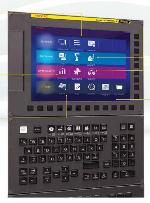
Machine collision avoidance Uniform tool information management for machine
