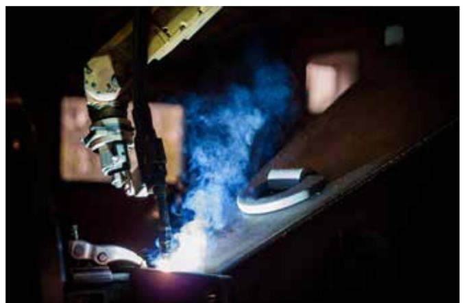
workpiece can be tacked. Sometimes, the ARC Mate robot from FANUC still needs a bit of support and oversight from Ronny Hahn.
