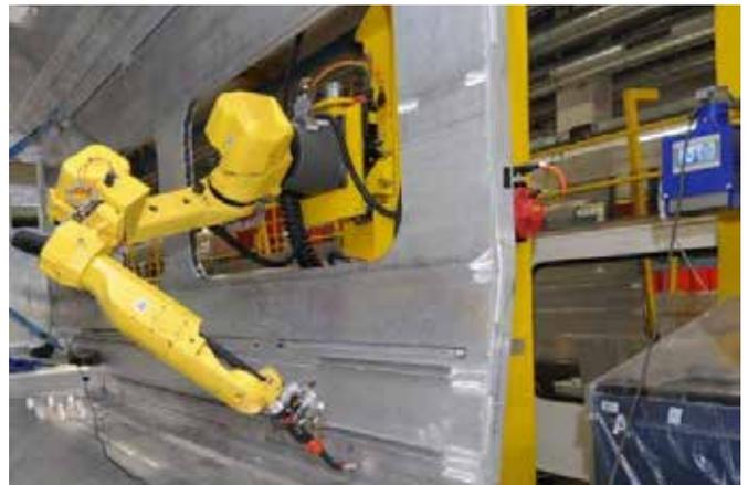
The robots are mounted on a platform, which is in turn sitting on a travel rail. Thus, the entire length of the vehicle body remains accessible. All chassis and travel axes are driven by high-precision steering racks and FANUC servomotors, which are easily integrated into the robot control as axes.
