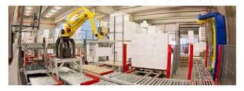
because June is a busy month). The end piece, the stacking robot, was put in standstill in August 2011 and successfully started up. The gain in speed on the packaging line is big, with this line one can manage 60 m³/hr and for some types up to 80 m³/hr, thus twice as much as earlier. The night shift can thus be dispensed with.
