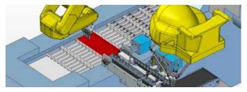
easily managed. We just need to intervene on the software to move all types of products. Our solution is totally universal and provides a significant benefit with regards to the compactness of the final system." The entire machine measures around 3 m and hosts 2 robots positioned in such a way as to allow easy operator access and to facilitate the periodic cleaning activities.
