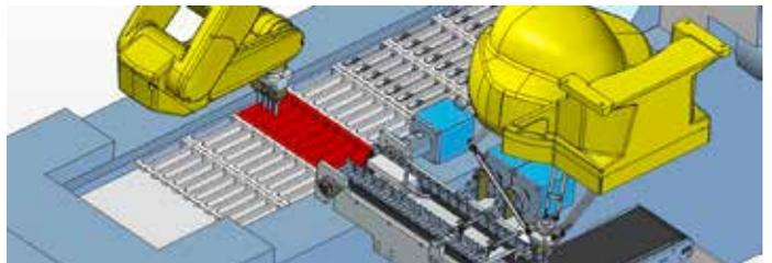
easily managed. We just need to intervene on the software to move all types of products. Our solution is totally universal and provides a significant benefit with regards to the compactness of the final system.” The entire machine measures around 3 m and hosts 2 robots positioned in such a way as to allow easy operator access and to facilitate the periodic cleaning activities.
