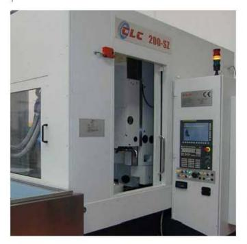
The range of the dimensions that can be processed with the CLC machines is very broad and goes from diameters of 100 mm to 2000 mm for the vertical axis machines and with modules of up to 30 mm, while for the horizontal axis machines, pieces with a diameter of up to 500 mm and a length of up to 3000 mm can be processed.
