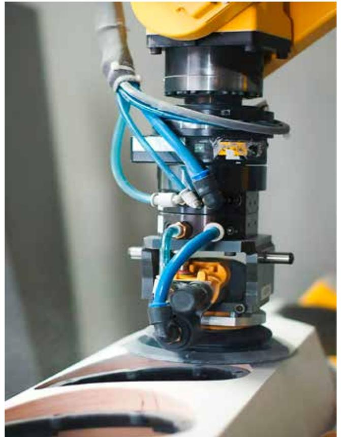
change the sanding heads as required, either during the process or at the end of the robot cycle. There is a total of six sanding heads within the cell, three on each side of the rotary table. The systems are also able to automatically change the sanding disks,
