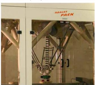
machine completely built by Robertpack, comprising 2x FANUC M3iA/6S robots for the box loading, underbox erector, tray edge closer and a lid setter. At the end of the line, a standalone FANUC M-710iC/70 robot palletizes the boxes. The BRC, IFS, Skal and HACCP certified company complies with the highest quality standards in the industry.
